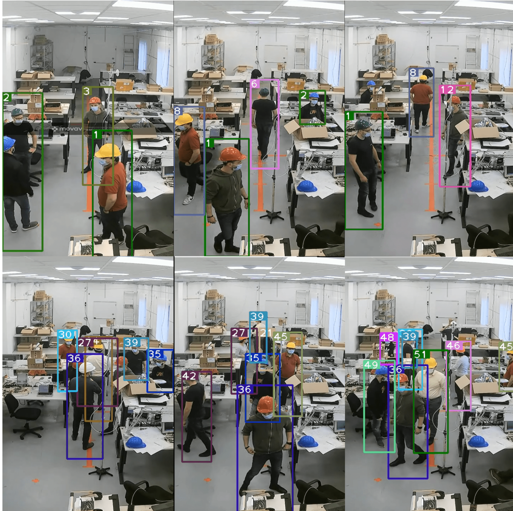
Figure 4.14: Final test done within the lab confirming the performance decrease due an increase of human detections.
