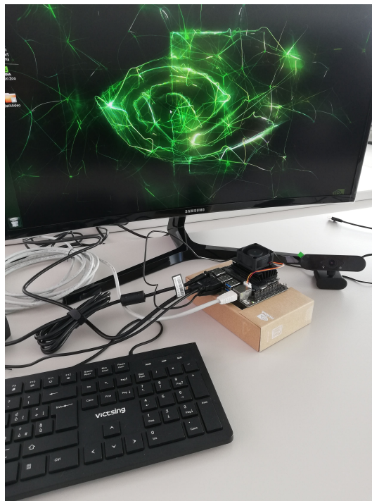
Figure 4.1: Experimental workstation setup and peripheral devices on Jetson Nano
