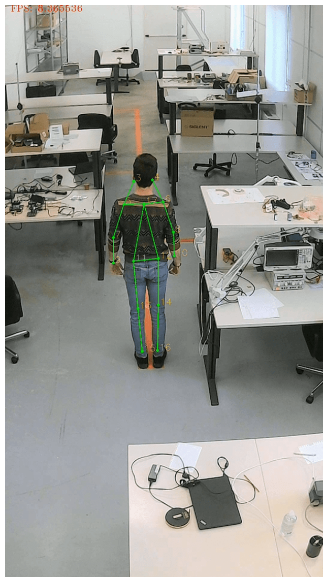
Figure 4.10: TrtPose tested in the laboratory up to 10 fps. Starting point of the path
