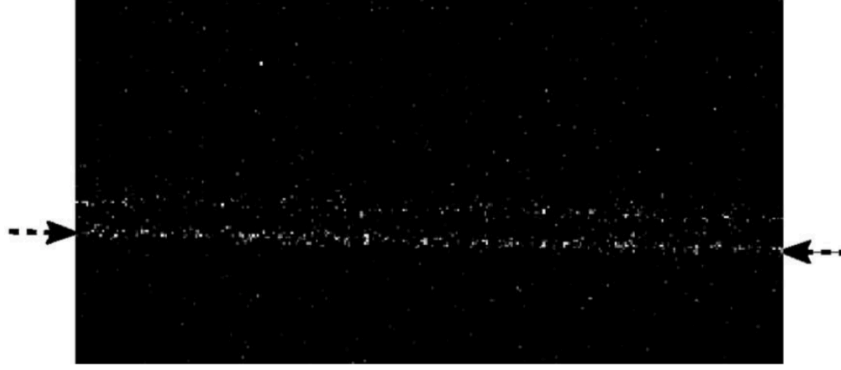
Figure 2.6: RIXS raw data. Typical image produced by the CCD detector during a RIXS experiment. Along the vertical direction we see the energy-related spatial coordinate, where photons have been diffracted by the grating. At the same time, photons with the same energy will hit the detector along iso-energetic lines perpendicular to the diffraction plane. This is shown in the horizontal direction as a degenerate spatial dimension over which we sum to obtain a spectrum. The two arrows indicate the presence of the zero energy-loss peak, i.e. the elastic peak. Figure from [42].
