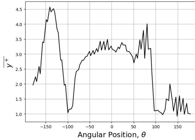
Figure 5.28: Non-dimensional Wall Distance y^+ , \Omega = 1 and Re = 5000
