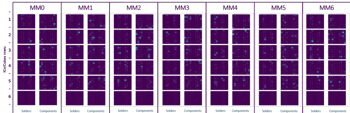
Figure 4.34: EWC distribution considering also the re-occurrences of same addresses, per TSOP, in both side of all memory modules matrix
