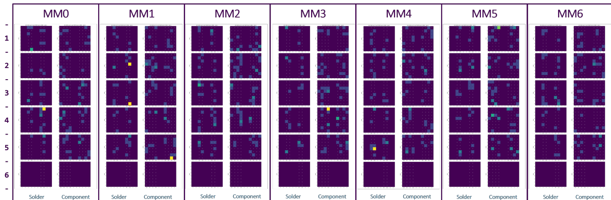
Figure 4.20: M-S EWC distribution per ICs/cubes and the relative TSOP levels in both side of all memory modules matrix
