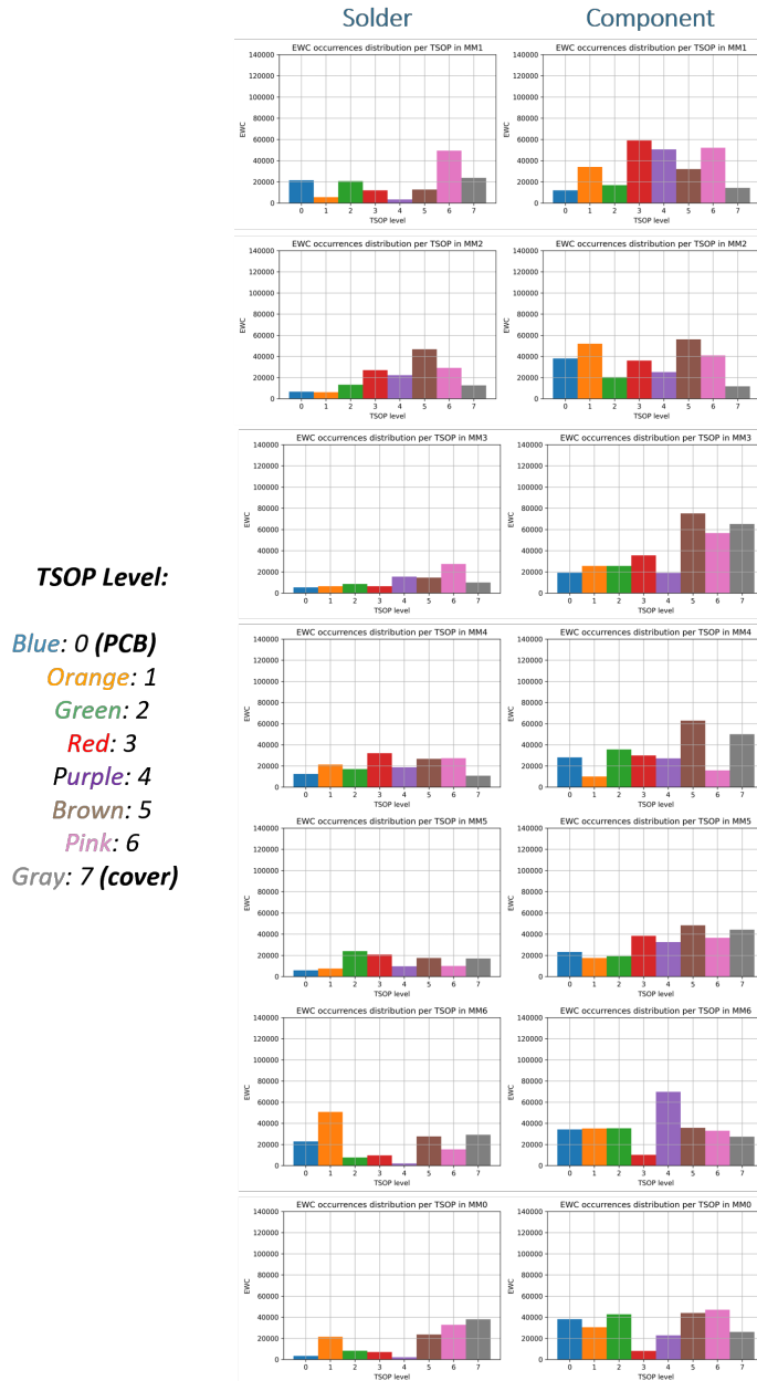
Figure 4.32: EWC occurrences distribution per TSOP in both side of all memory modules
