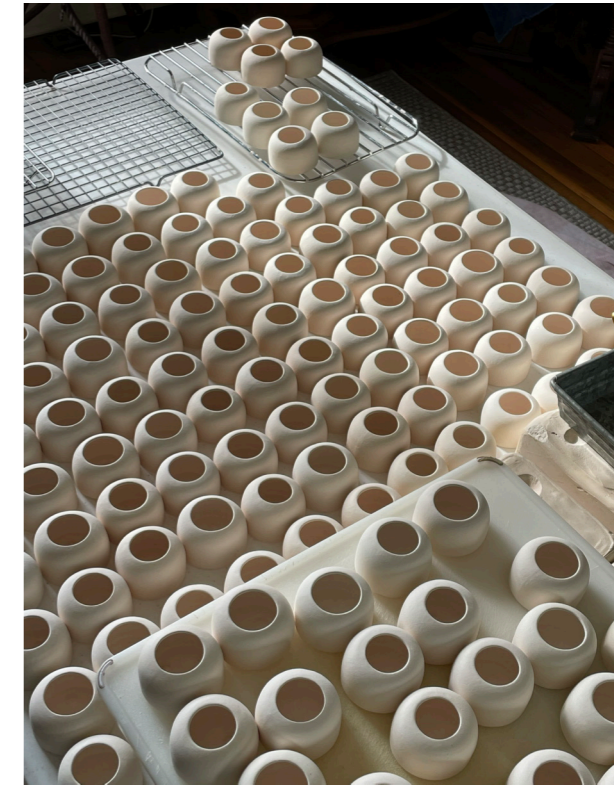
Fig.11: Slip casting production 2022 Shipleigh Goods
