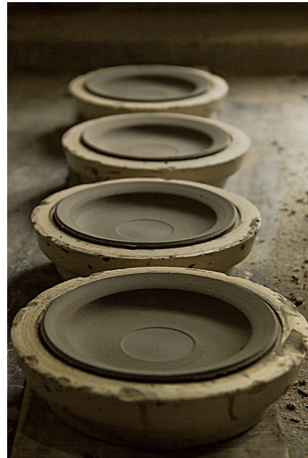
Fig.09: Press molded plates drying in plaster molds in Kurja, India Ankana Sen
