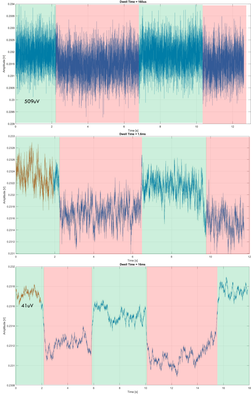
Figure 4.10: Output traces of a balanced experiments with \beta -carotene in toluene sample. Red boxes: Stokes OFF, Green boxes: Stokes ON. 160 \mu s dwell time and 509 \mu V standard deviation (top), 1.6 ms dwell time and 195 \mu V standard deviation (middle), 16 ms dwell time and 41 \mu V standard deviation (bottom).
