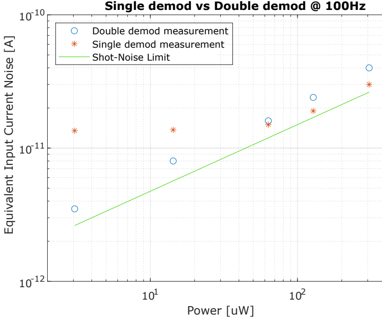
Figure 4.4: Fixed bandwidth equivalent input current noise at various input optical powers for single and double demodulation operations. In green the shot noise limit.
