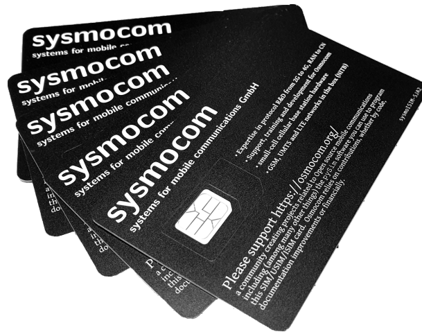
Figure 3.1: SYSMOCOM SYSMOISIM-SJA2 programmable SIM cards
