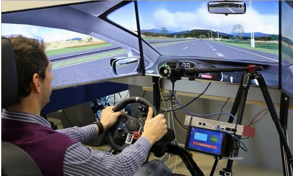
Figure 6.2: The proposed rPPG system tested in a driver simulator developed by General Motors.
