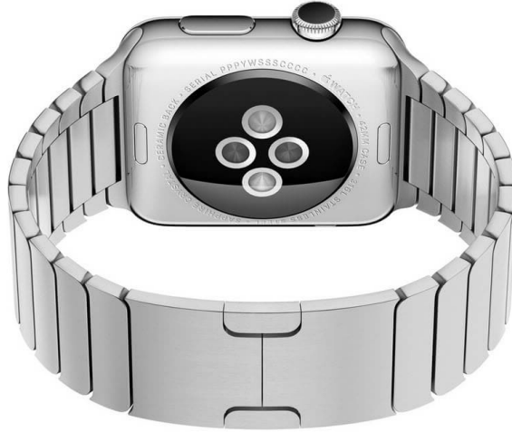
Figure 2.5: Rear view of a modern commercial wearable device (smartwatch) equipped with a PPG system.
