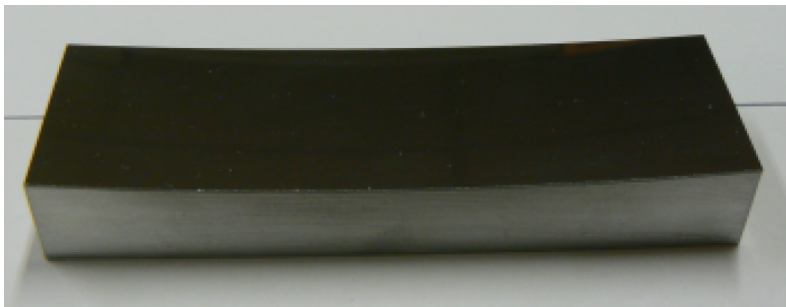
Figure 1.4: A Johansson-type bent crystal [6] .
