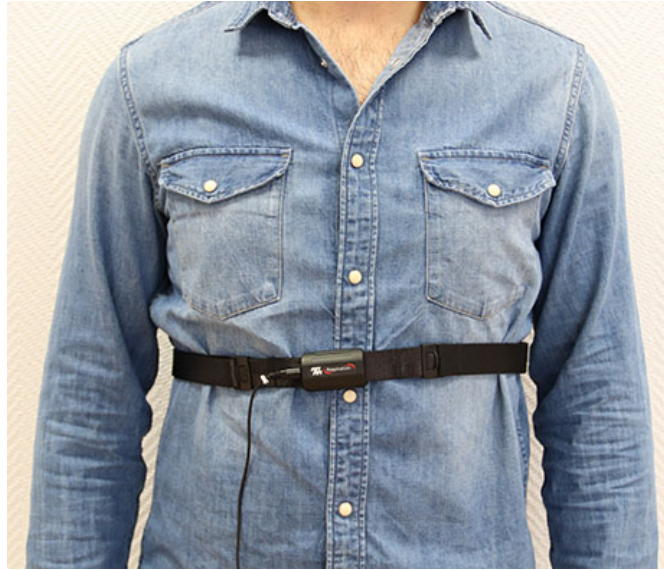
Figure 4.8: The placement of a respiratory belt around the thorax [140]
