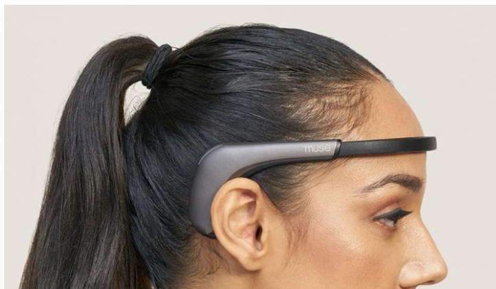
Figure 3.1: A wearable headband device for EEG acquisition, model Muse 2, https://choosemuse.com/
