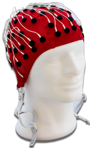
Figure 4.5: An example of an EEG cap with 61 electrodes and a strap [5]
