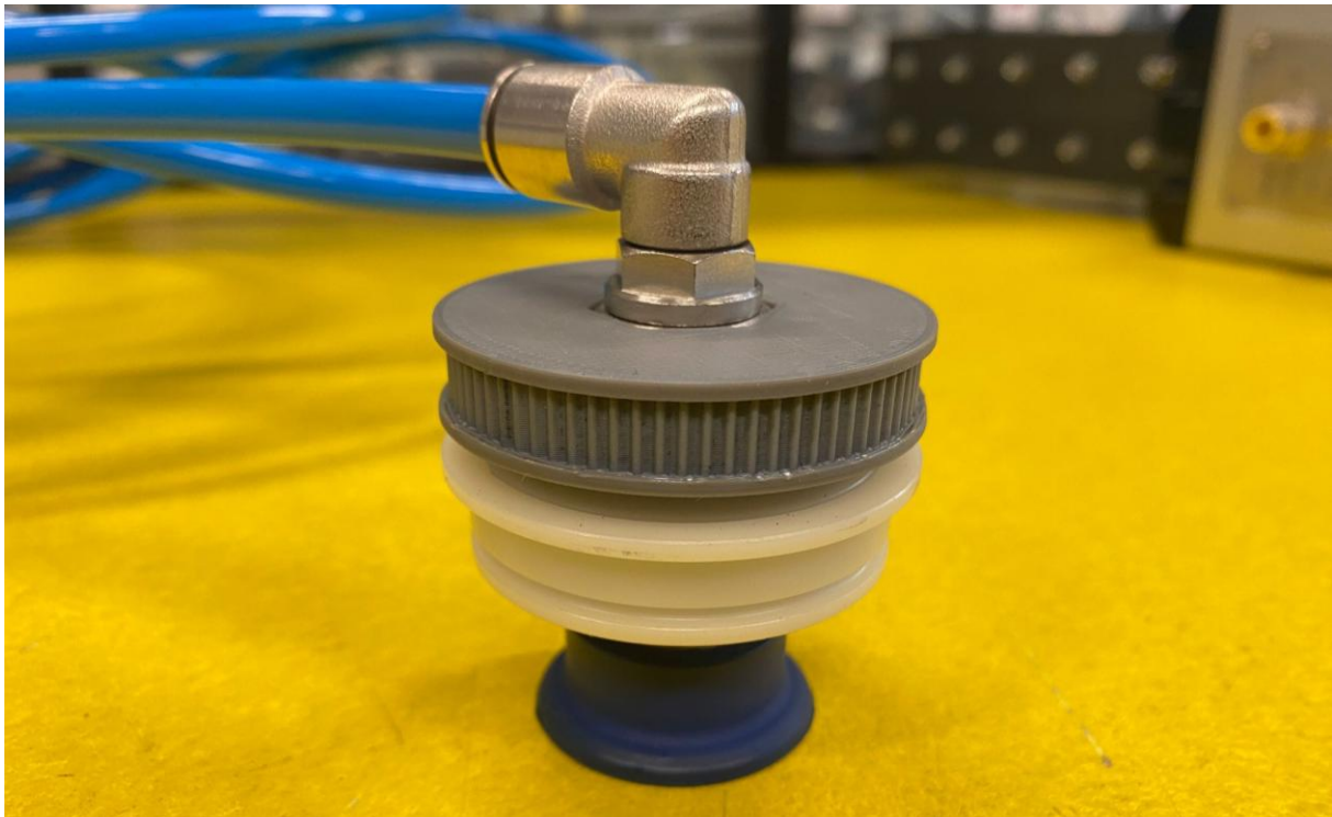
Figure 3.14: Pneumatic swivel fitting, suction cup and 76 tooth pulley
