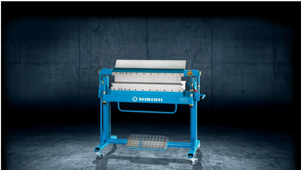
Figure 3.18: Schechl UK 100 S bending machine
