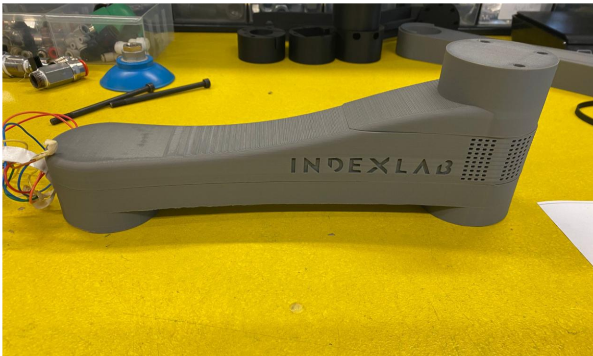
Figure 3.5: Custom 3D printed end effector
