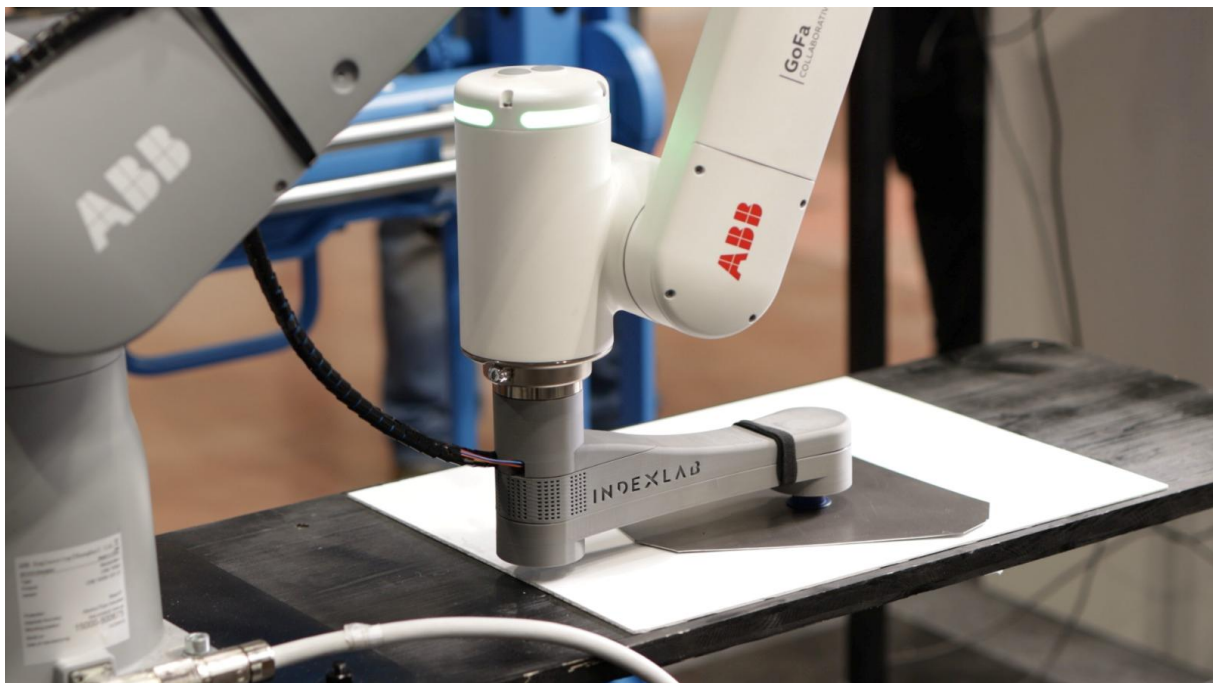
Figure 3.10: Metal sheet pick-up operation at CaseItaly 2026
