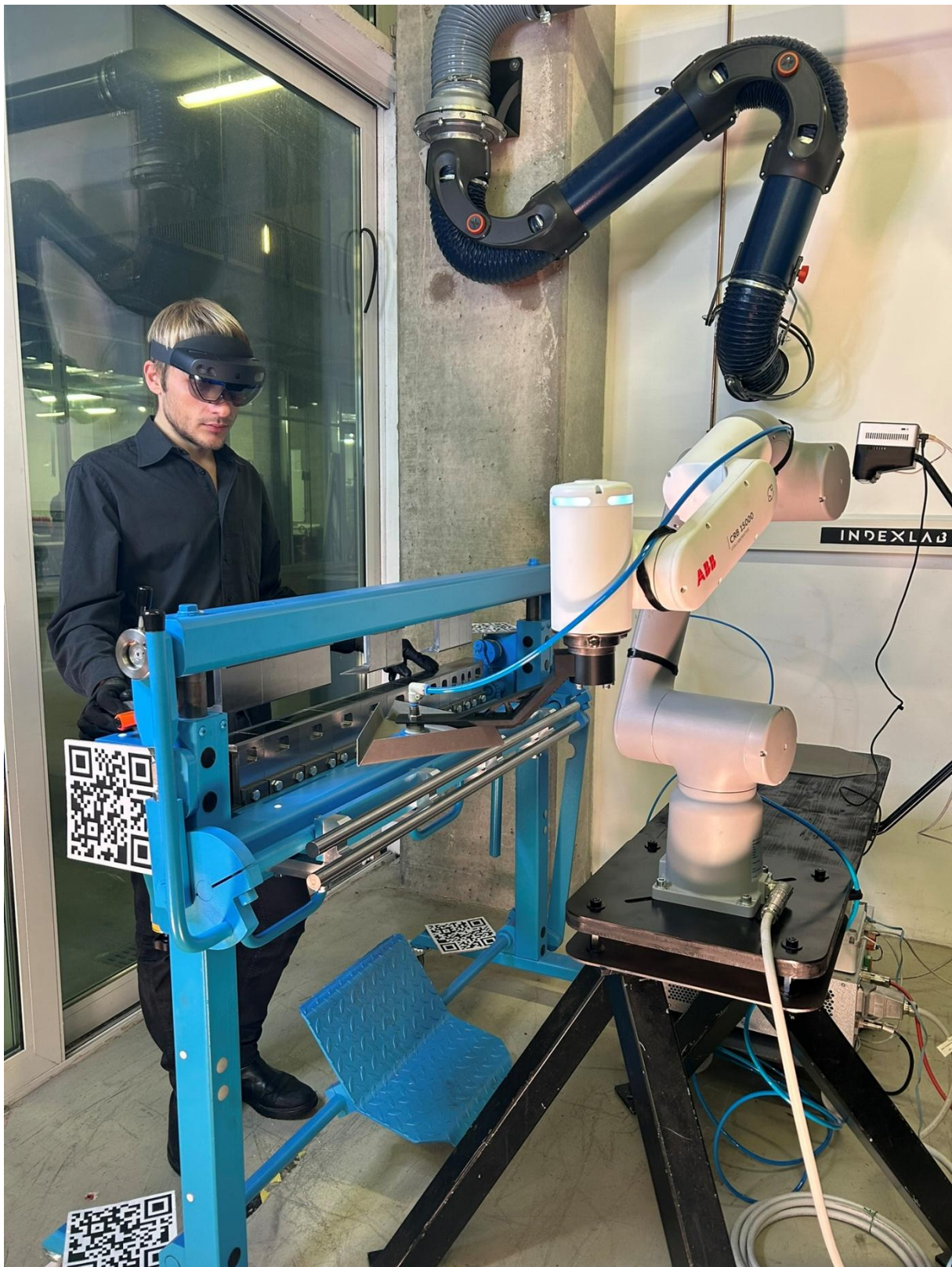
Figure 3.2: Robotic sheet metal handling at Indexlab
