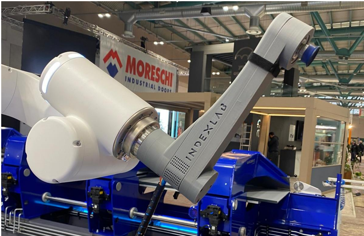
Figure 3.9: End effector mounted on Gofa 5
