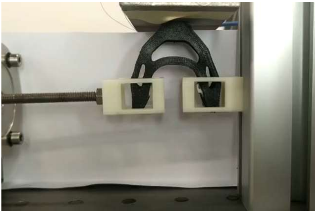
Figure 124 - The ad-hoc set-up designed to test the devices with a closed-loop control of the gripping force exerted. A load cell (left side of the image) and a pair of special fixtures 3D printed in ABS with adjustable distance were used.
