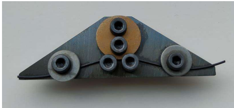
Figure 115 - Jig used for heat treatment of SMA spring. The wire loops around the brass disc and the tails are formed and held fixed by bolts and washers.
