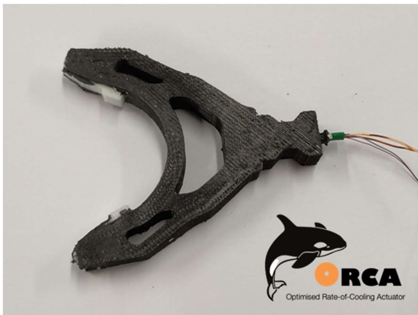
Figure 123 - Orca: “Optimised Rate-of-Cooling Actuator”, displaying the black modified PDMS matrix used for the body, cast over the plain stiffer white PDMS used to cover the electric connections in the tails.
