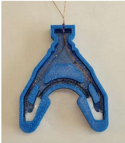
Figure 121 - Insertion of the parts created in the first step into the second mould that forms the body of the actuator.
