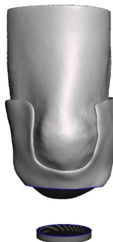
Figure 6.7 Removal of the upper part of the cylinder and the lower part of the socket
