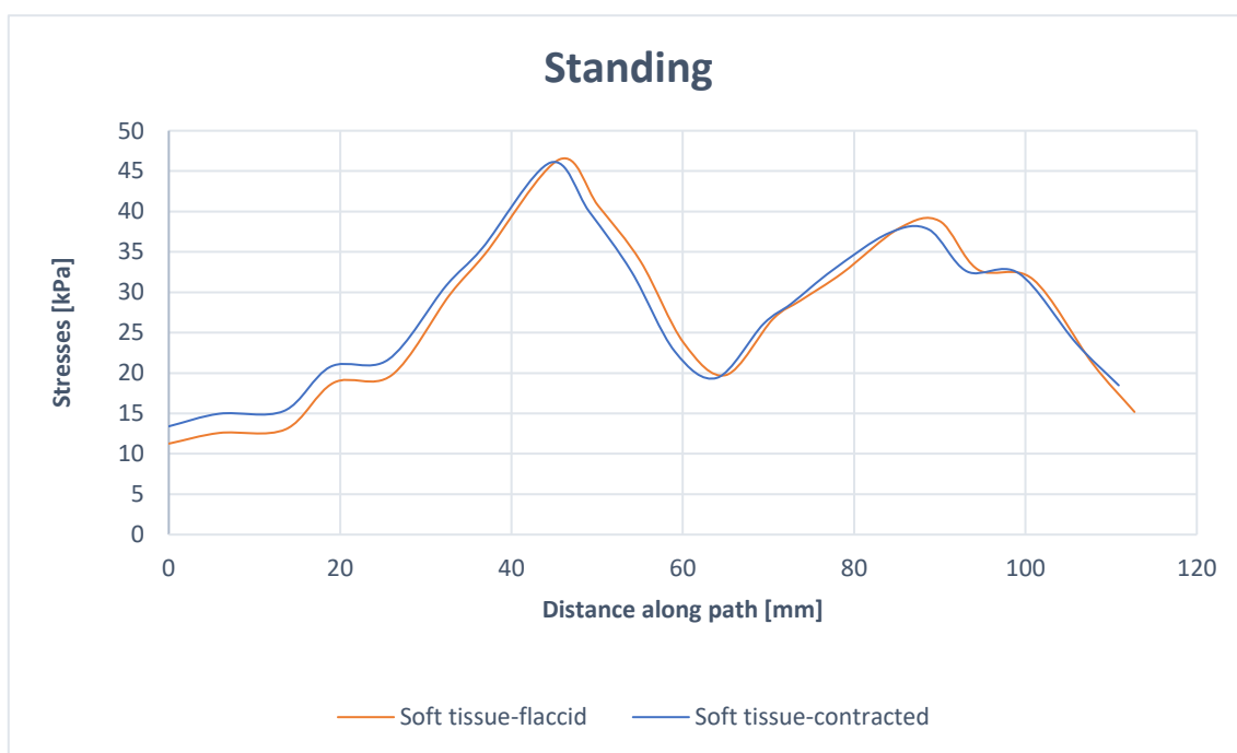
Figure 8.22 Comparison of Von Mises stresses along the path in double leg standing with flaccid soft tissue and contracted soft tissue
