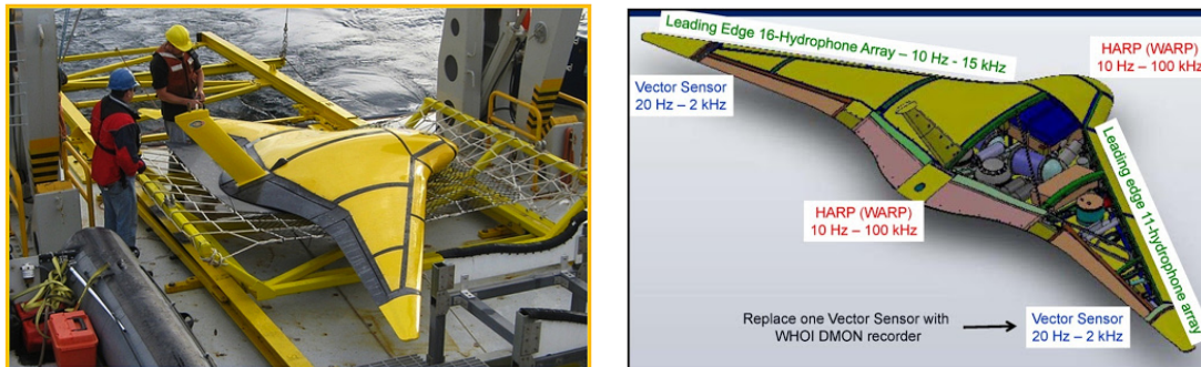
Figure 1.6: Liberdade ZRay in deployment and CAD of its inner components.
