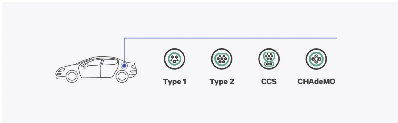
Figure 2 - Types of charging connectors
