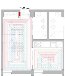
Plan of the floor heating system for a typical span of the Convitto SCALE 1:50
