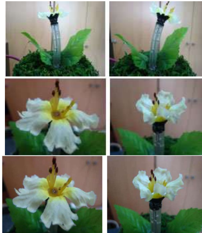
Figure 13 - SMA actuated flower robot
