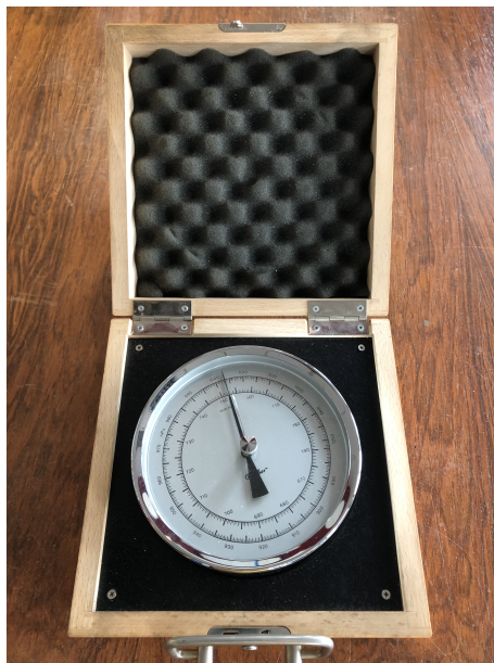
Figure 5.4: Barometer used for atmospheric pressure measurement
