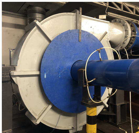
Figure 2.7: Case of centrifugal compressor
