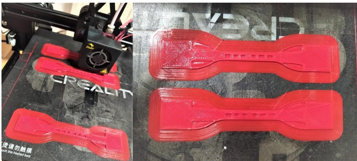
Figure 26 Tensile specimens optimised sections during printing
