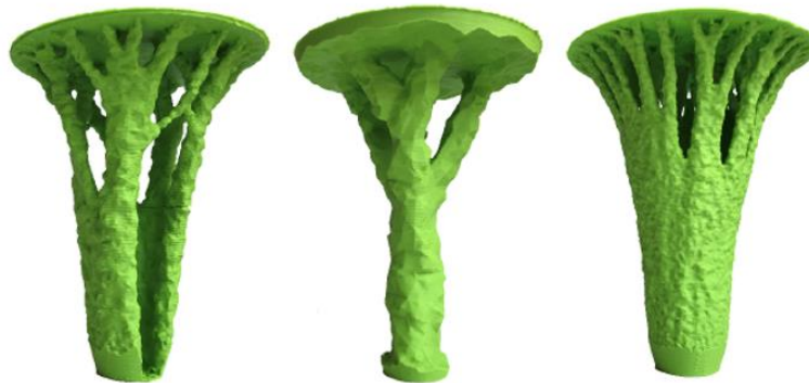
Figure 11 3D printed samples from topology optimisation [15]
