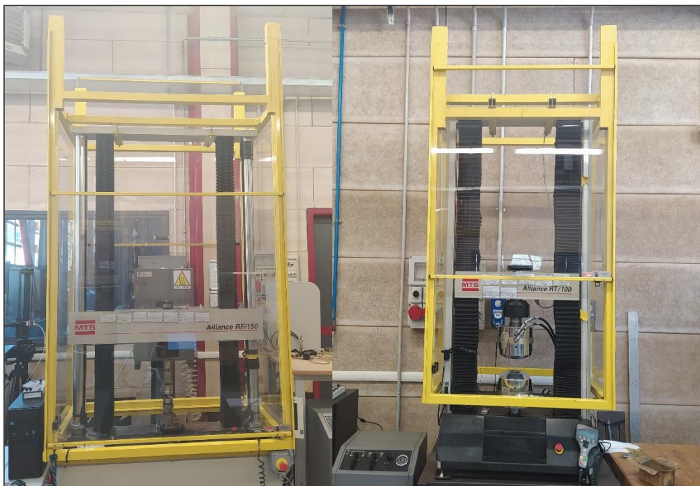
Figure 32 Compression and Tensile testing machines
