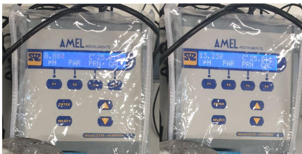
Figure 43 pH test for the water used before and after washing with suction filtration.
