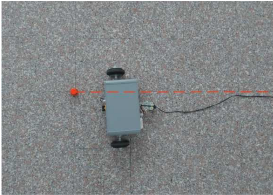
Figure 5.8: Straight movement experiment showing the displacement error.
