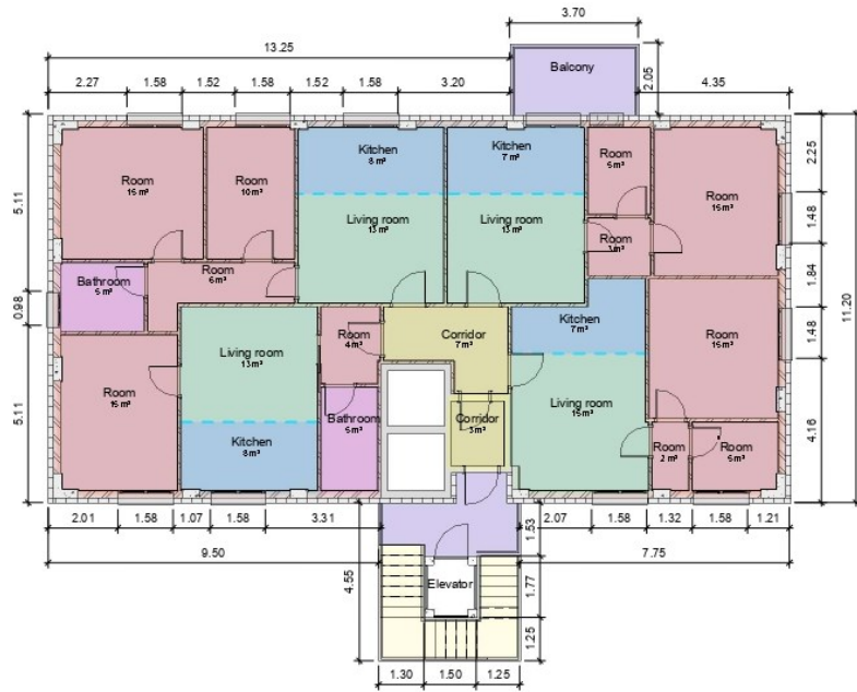
Figure 18: 3rd Floor plan
