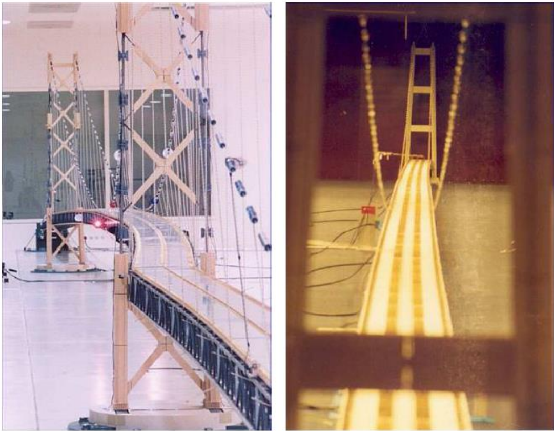
Figure 1.25: Comparison of Akaishi-Kaikyo (left) and Messina (right) horizontal deflection due to wind in the wind tunnel.
