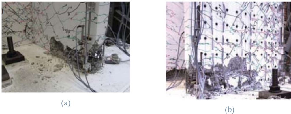
Figure 3.15 Failure of the East Flange TUC (Distributed Reinforcement) (Constantin & Beyer, 2016)
