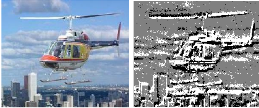
Figure 14: To the left a standard camera image, to the right a grayscale view of an event based image of the same scene with positive events represented as white pixels and negative events represented as black pixels. Another common choice is blue for negative events and red for positive events. Images taken from the Caltech101/N-Caltech101 dataset [34].
