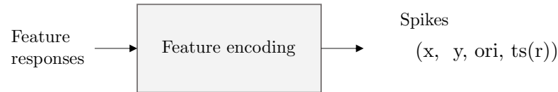
Figure 46: Feature encoding. The spike timestamp ts depends on the feature response value r . (cfr. Section 2.3.2)
