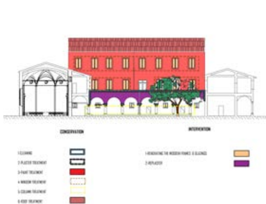
Conservation project_ Interventions on the existing CONSERVATION/INTERVENTION
