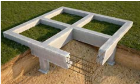
Fig. 04.4: Monolithic strip foundation
