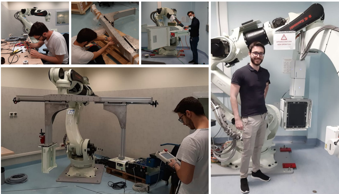
Figure 6.1: The development of the CBCT imaging system in testing room (left). The final CBCT imaging system after installation (right)
