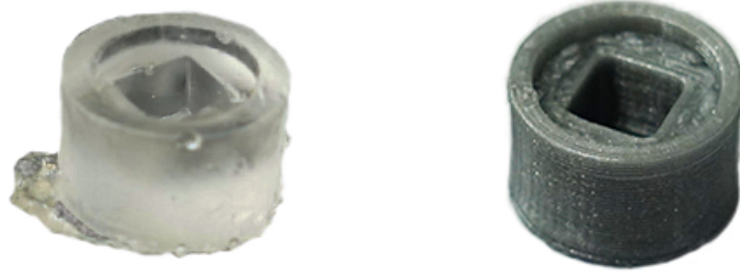
Figure 3.1: Endcaps comparison. On the left the old epoxy-resin one with some defects and residual scrap, while on the right the new 3d-printed PLA one, showing excellent finishing and geometrical precision.
