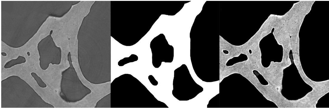
Figure 2.10: Image filtering process: focus on non-filtered image (left), the applied binary mask (center) and the final processed image (right).
