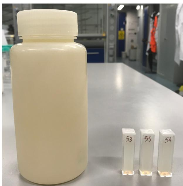
**Figure 23.** Volumetric cylindrical phantom containing PAGAT gel composition next to three spectrophotometric cuvettes as comparison. External phantom dimensions: 75 mm base diameter, 134 mm height to the shoulder, 57 mm lid diameter, 165 mm total height.
