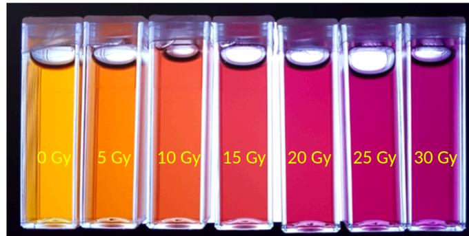
**Figure 1.** Photograph of Fricke gel dosimeters irradiated up to 30 Gy at 5 Gy increments [31].
