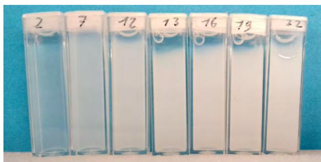
**Figure 2.** Photograph of PAGAT polymer gels irradiated at increasing doses from left to right.
