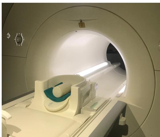
**Figure 26.** Phantom in the automatized bed for MRI scanning.
