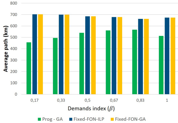
Figure 6.8: Comparison of Average Path Lengths in the Italian 10 nodes topology between P-FON and FON solutions.
