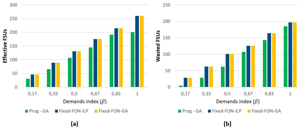
Figure 6.7: Comparison of Effective (a) and Wasted (b) FSUs consumptions for the Italian 10 nodes topology between TE P-FON and Given Trees FON
