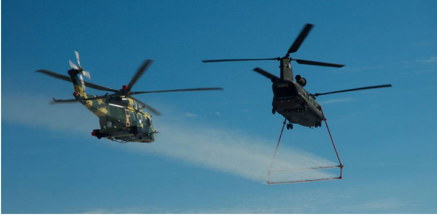
Figure 1.1: AgustaWestland’s AW189 icing trials of full icing protection system. [7]
