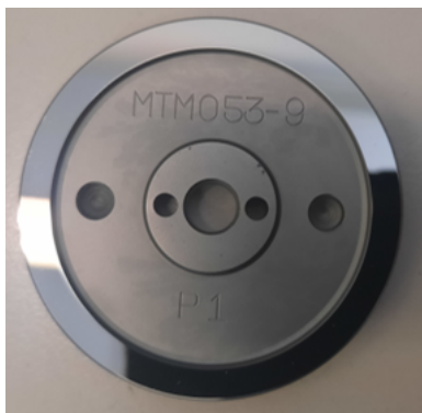
Figure 2.4: Picture of the AISI52100 standard MTM sample.
