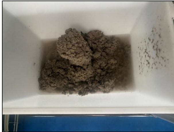
Figure 14: Solid fraction discharged from the disc filtration unit.
