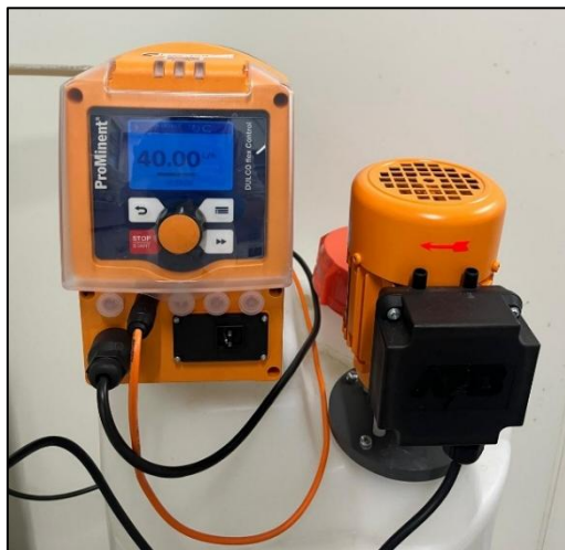
Figure 18: Peristaltic pump operated at the selected reference flow rate.
