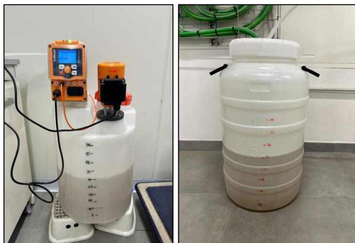
Figure 19: Feed tank (left) for influent sampling before filtration and the filtrate tank (right) for sampling after passage through the filter medium.
