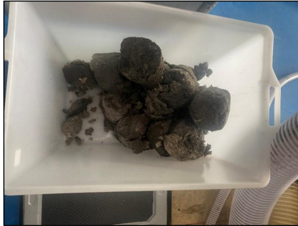
Figure 17: Solid fraction discharged from the belt filtration unit.
