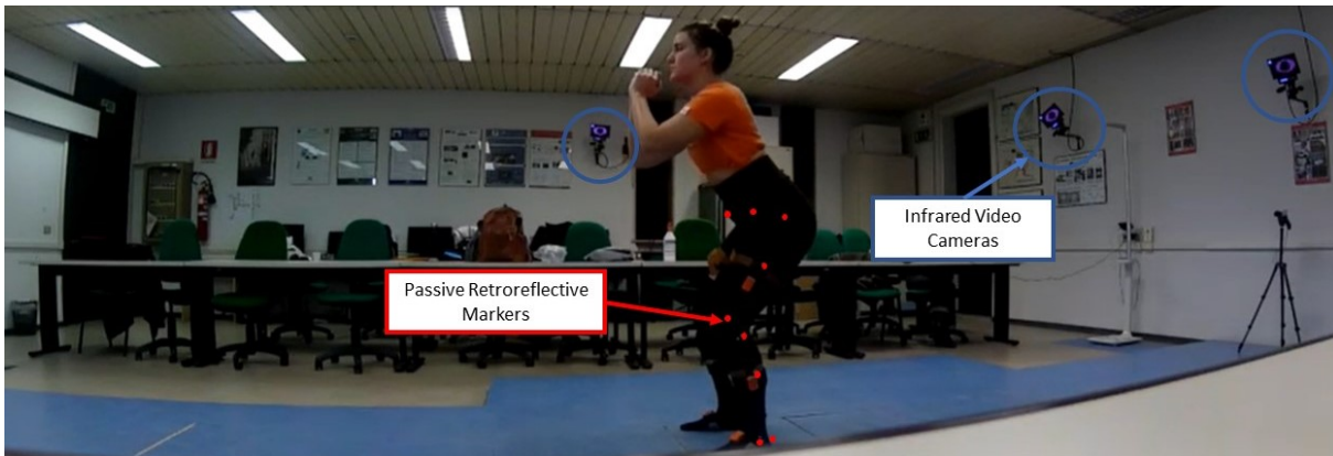
Figure 2.2: Representation of the MOCAP using external markers placed on the body surface
