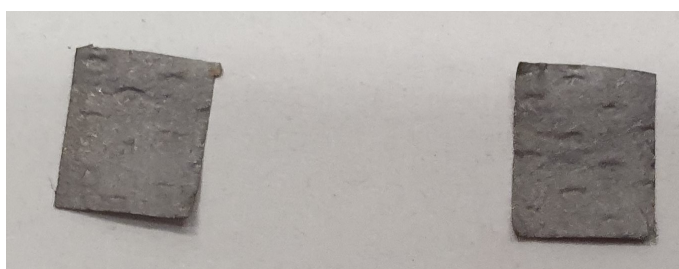
Figure 3.10: Two dried substrates produced by centrifugation.
