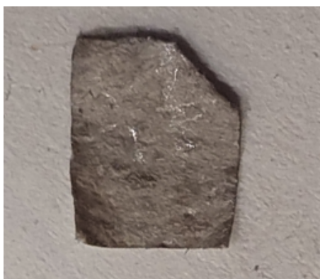
Figure 3.11: Example of the one-corner truncated rectangular shape adopted for the production of the SERS substrates by centrifugation.
