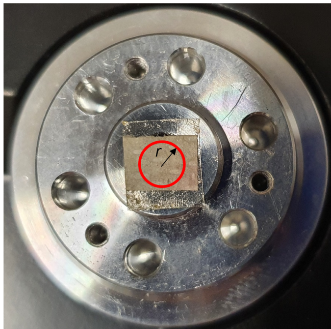
Figure 4.3: The substrate is mounted at the centre of the rotating device and the laser is kept fixed at distance r from the rotation axis. During the SERS measurement, the laser track on the substrate describes an annular surface (in red).
