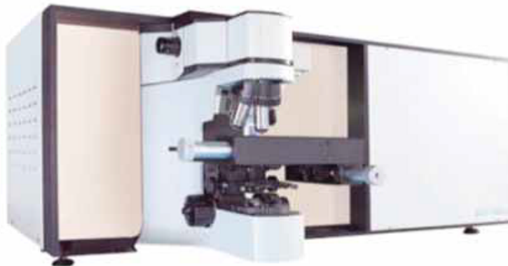
Figure 4.1: The Horiba Jobin Yvon LabRAM HR8000 used to acquire spectral data (taken from [8]).
