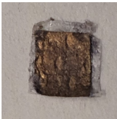
Figure 7.14: SERS substrate obtained by natural sedimentation of concentrated Au colloid after incubation and drying.
