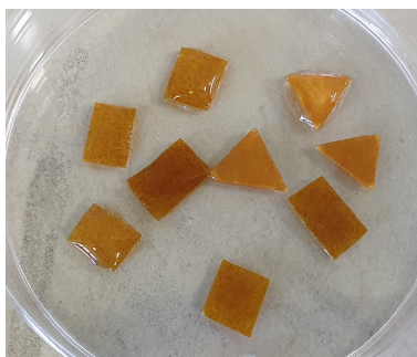
Figure 7.3: SERS substrates produced by direct paper reduction, without TSC.
