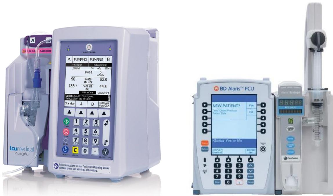
Figure 32 – Volumetric (left) and syringe (right) infusion pumps (source: ECRI)
