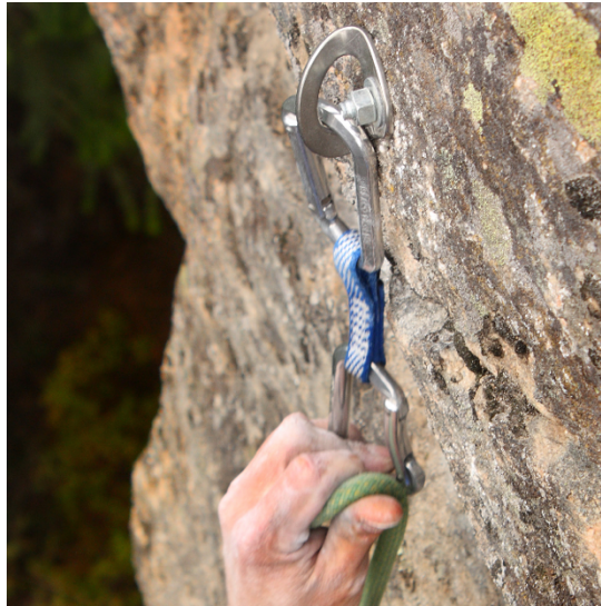
Figure 8 Anchor fixed in the rock
