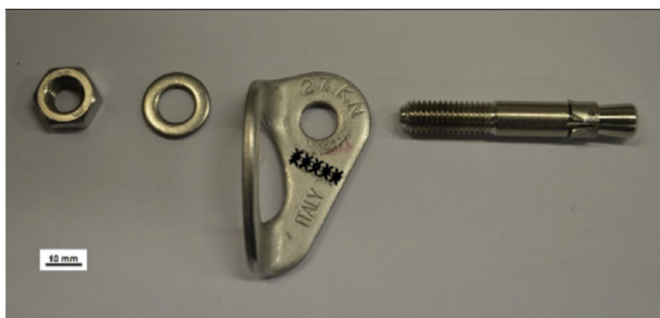
Figure 6 Components of an expansion bolt
