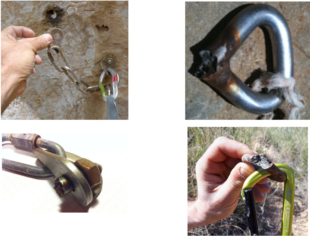
Figure 9 Examples of failure of rock anchors
