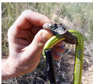
Figure 2 Example of rock anchor failure
