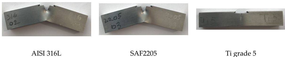
Figure 46 – SE(B) specimens after the fracture toughness tests.
