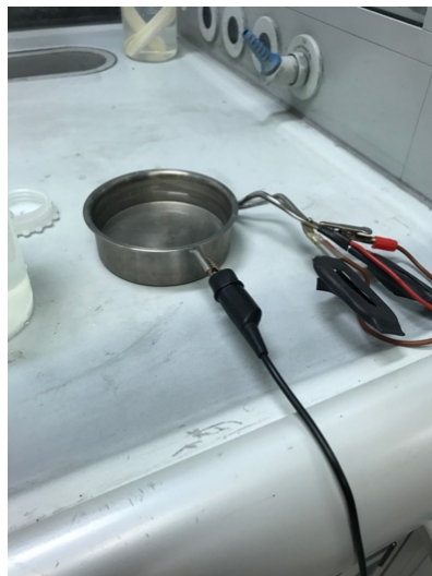
Figure 17 Electrochemical etching with oxalic acid
