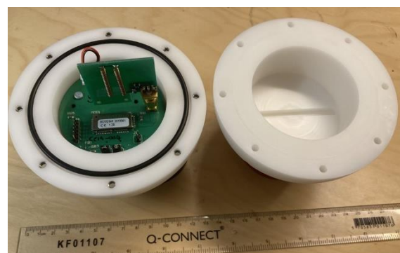
Figure 5: Cryoegg probe, made of two halves of machined acetal copolymer sealed with an O-ring and eight machined screws [13]
