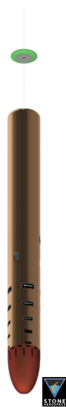
Figure 1: Concept of a Cryobot with an RF communications puck deployed for Ocean World exploration.
