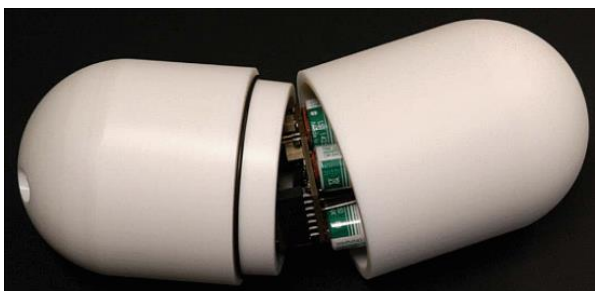
Figure 4: Glacsweb probe, with electronics and sensors housed in a 68 mm diameter plastic egg-shaped capsule made of two halves permanently bonded [12]
