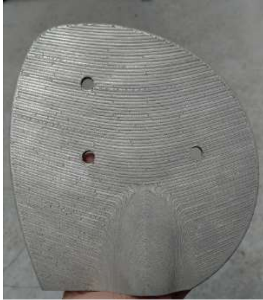
Figure 6-20 Final part after removing the supports courtesy by Add Italia.
