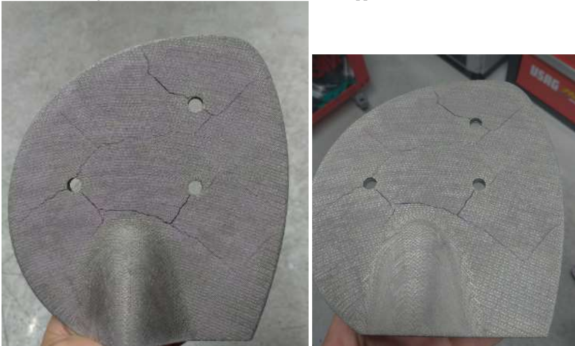
Figure 6-21 Cracks occurred on the final part courtesy by Add Italia.
