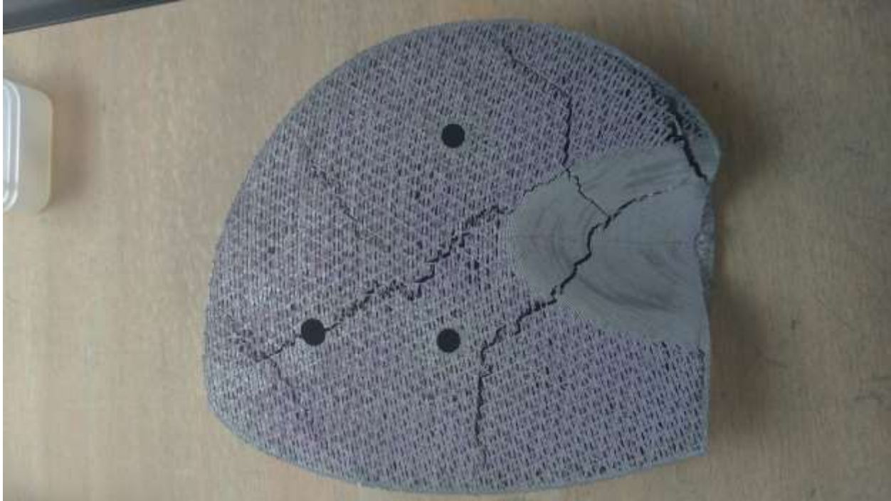
Figure 6-22 Cracks on support structures courtesy by Add Italia.
