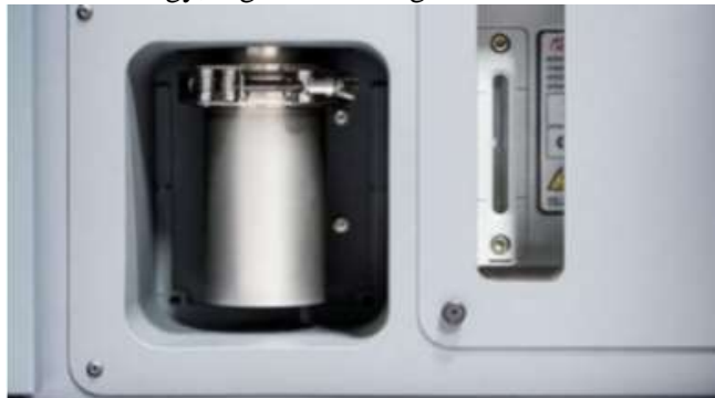
Figure 3-11 Binder trap for collecting and removing remaining binder of the part [23].
