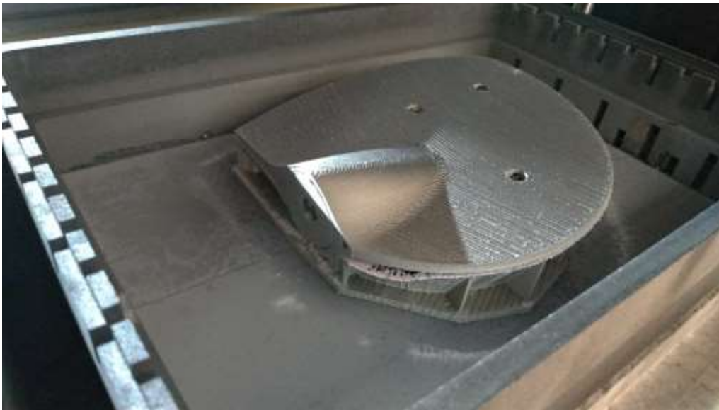
Figure 6-19 Part after sintering process with supports courtesy by Add Italia.
