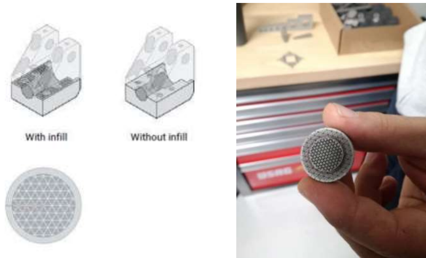
Figure 3-13 Left side shows Cross sectional thickness based on wall thickness and internal infill [40] and Right side shows Example of internal infill of a part. Courtesy of Additive Italia Srl.
