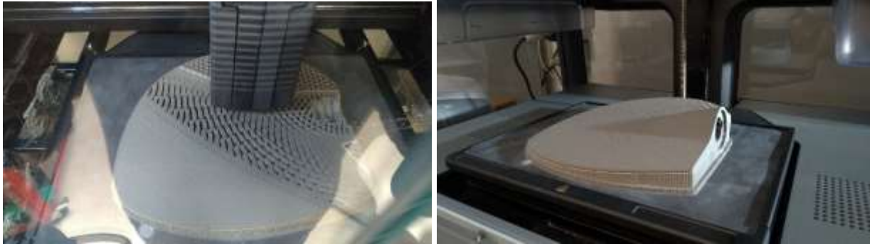
Figure 6-10 Left side shows blade while printing and Right side shows final printed part called as green part courtesy by Add Italia.
