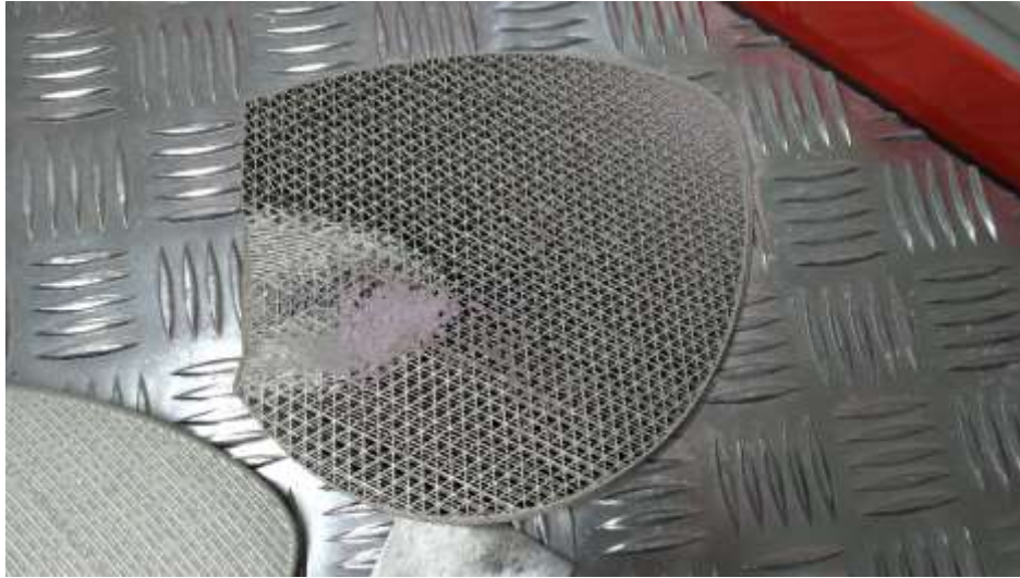
Figure 6-12 separated supporting structures of blade courtesy by Add Italia.
