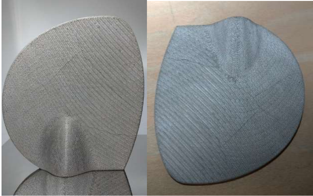
Figure 6-14 Cracks on the blade courtesy by Add Italia.
