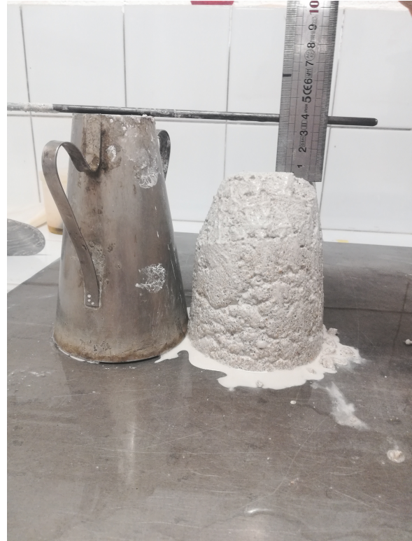
(b) Slump composition CaO 10% w/l reduced
