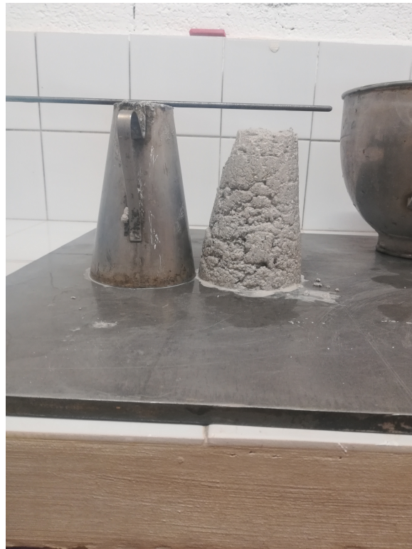
(c) Slump composition MgO 5% + CEMI 5% w/b reduced
