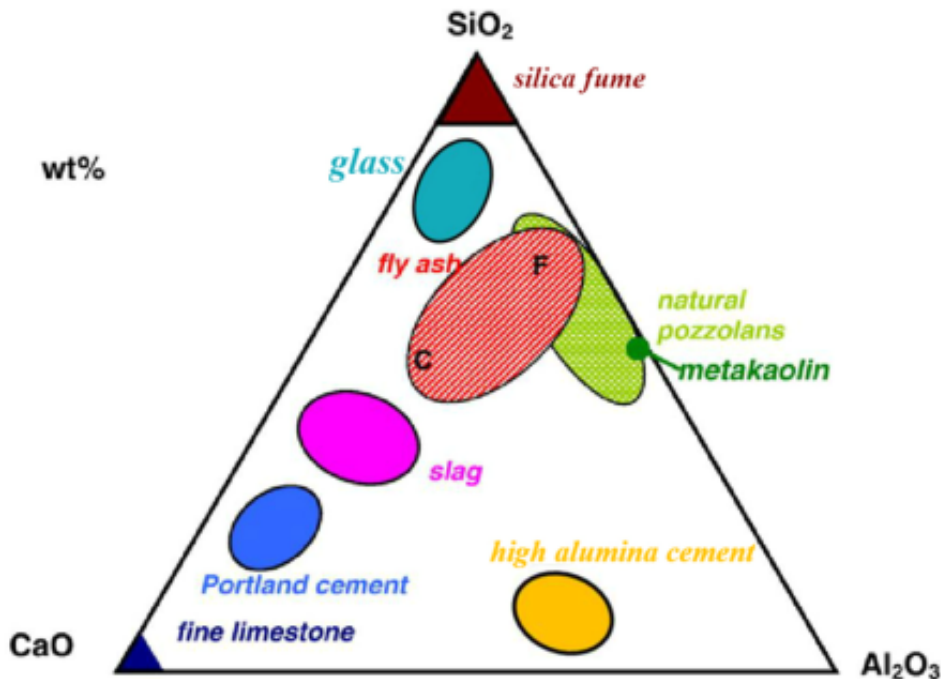
Figure 2.1: CaO-Al 2 O 3 -SiO 2 ternary diagram (wt% based) of common cementitious materials [25]
