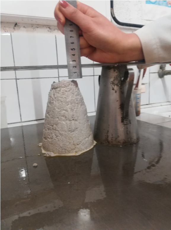
(a) Slump composition CaO dried 10%
