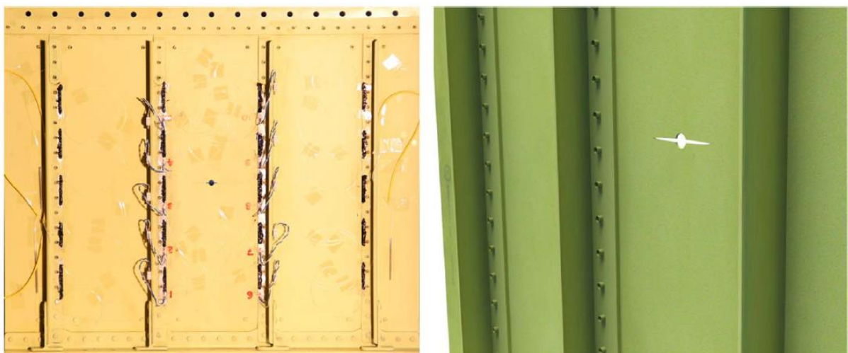
Figure 9. Experimental setup for fatigue damage testing. [16]
