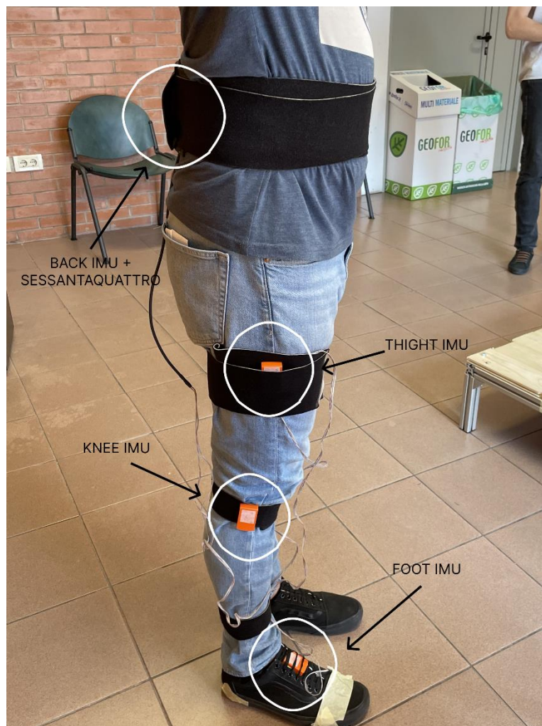
Figure 17, placement of the four IMUs and the Sessantaquattro on one of the subjects.
