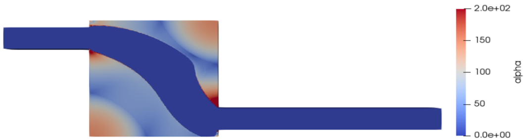
Figure 5.4: Topology optimization result
