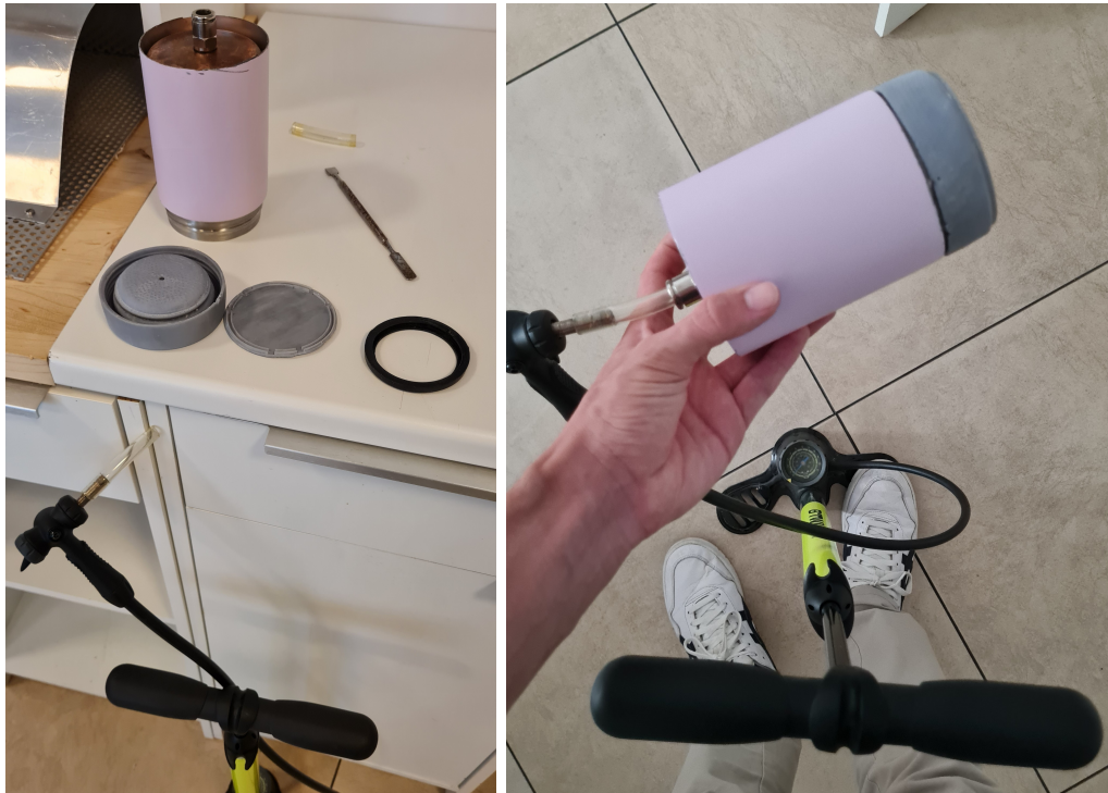
Figure 4.11: Pressure test rig presented and assembled
