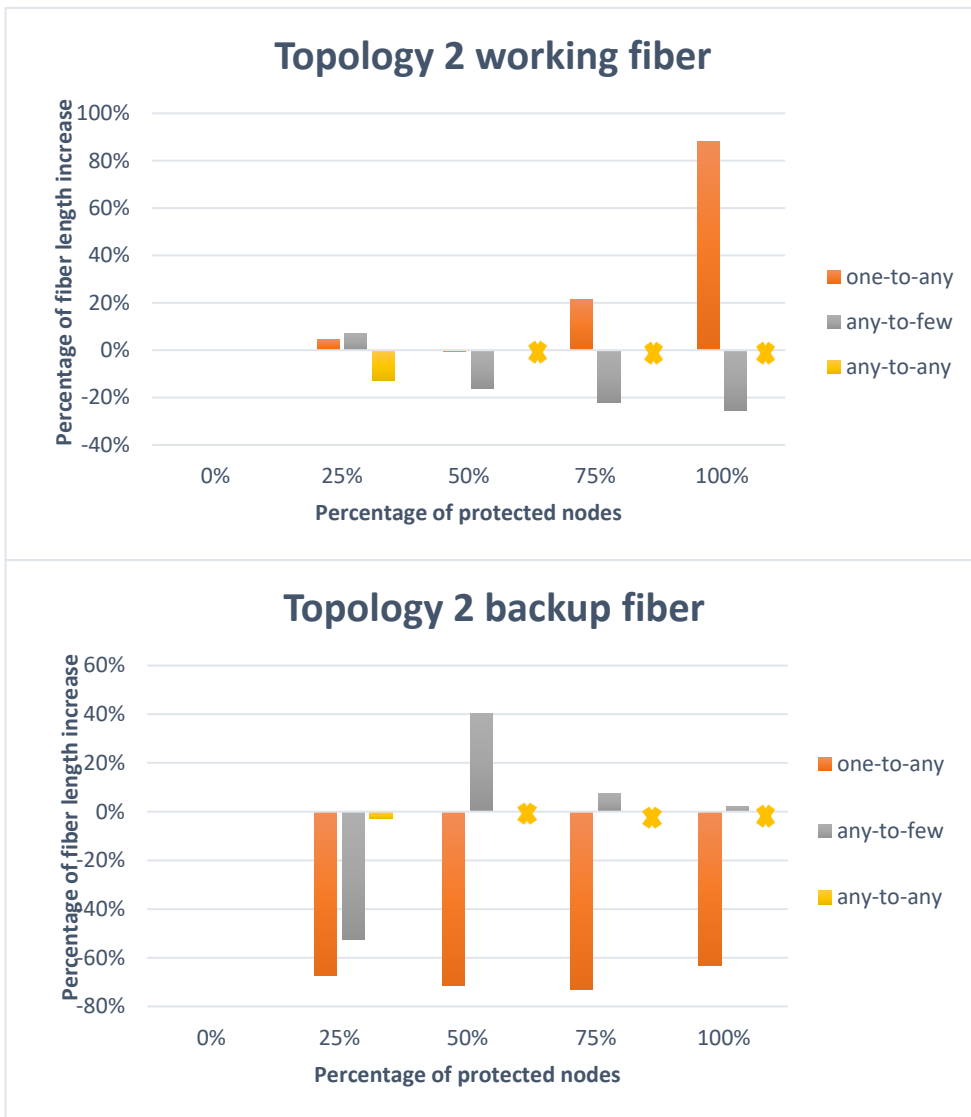
Figure 21. Total working and backup fiber length increase for topology 2 in different local interconnects and different % of protected nodes with ONU-ONU protection with respect to RN-ONU protection
