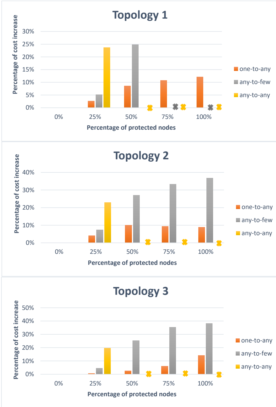
Figure 19. Trenching cost increase for the three topologies in different local interconnects and different % of protected nodes with ONU-ONU protection with respect to RN-ONU protection
