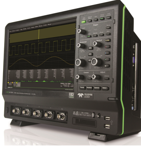
Figure 3.7: The Teledyne LeCroy HDO6054 high-definition digital oscilloscope used as the benchmark data acquisition system for offline multi-heterodyne signal processing.
