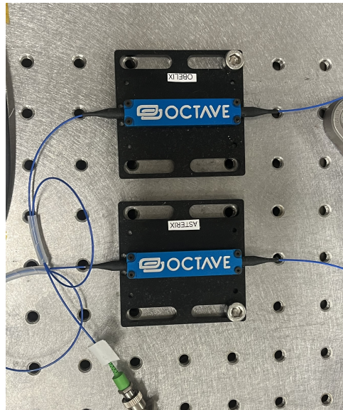
Figure 3.3: Commercial supercontinuum generation module (Cosmo by Octave Photonics) used in the experimental setup.
