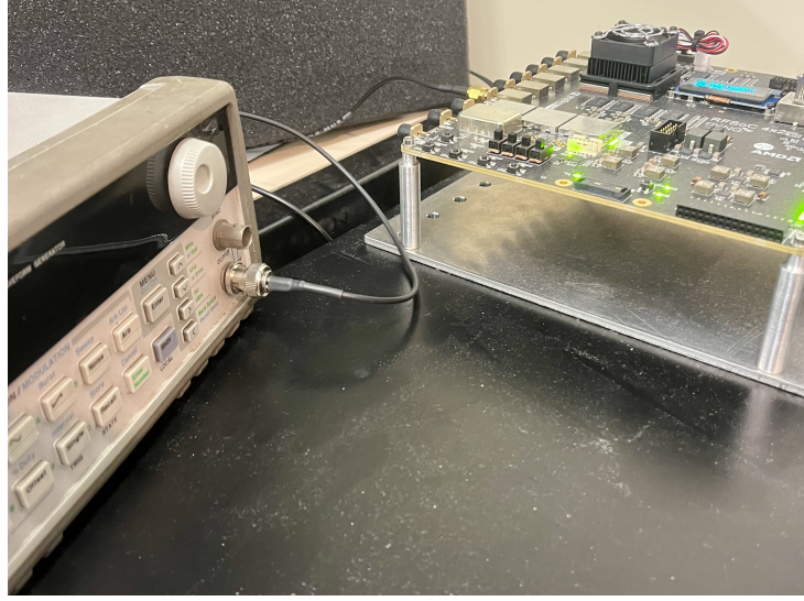
Figure 5.4: Laboratory experimental setup with the external Hewlett Packard 33120A waveform generator connected via SMA cable to the RFSoc 4x2 receiver channel input.
