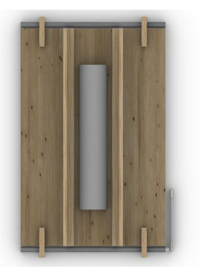
Cut the fiberglass mesh to obtain a strip that is two and a half times the length of the base and 5 cm wider than the width of the tracks.
