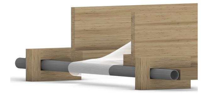
Place the cut mesh at the rear tube, as shown in the figure, in order to obtain two equal-length ends. Once positioned, ensure that the underlying formwork is clear to proceed with the next step.
