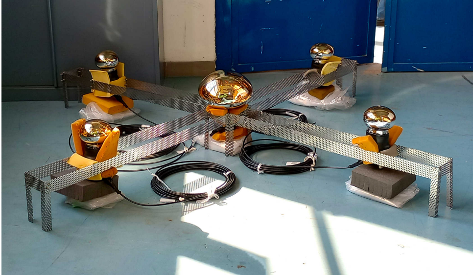
Figure 4.4: Test assembly of the PMT holder (before reinforcement of the cross arms).
