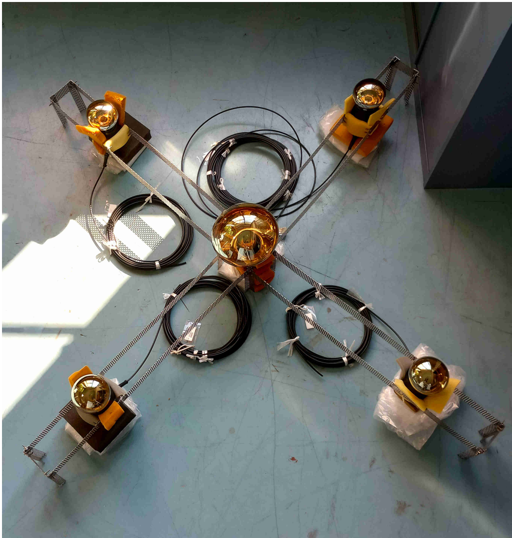
Figure 3.13: Holding test of cross holder using the 5 PMTs of the reference configuration.
