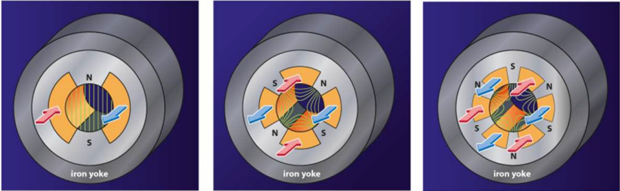
Figure A.2: Dipolar (left), quadrupolar (center) and sextupolar (right) superconducting magnets (Courtesy of Lucio Rossi).
