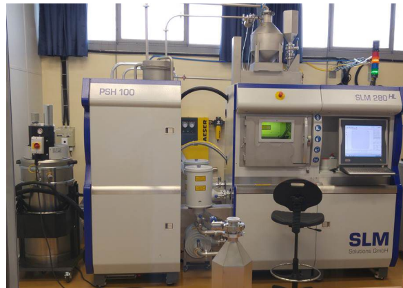
Figure 6.8: Additive manufacturing machine (SLM 280) at CERN (Courtesy of Romain Gerard).
