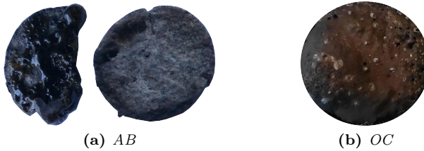
Figure 4.7.: Alkali basalt (a) and ordinary chondrite (b) samples after plasma exposure. In the former (a), glassy features formed after the resolidification. In the latter (b), the change of colour, probably a sign of the change in the oxidation state of iron, is visible.
